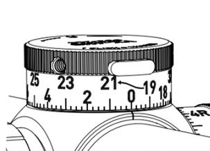
CDS-ZL2 Elevation Dial (locked position)
